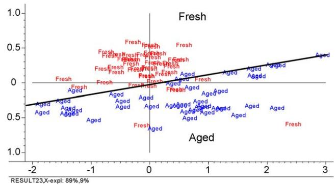
Fig. 2. PCA plot based on the six reference air corrected sensor readings from the on-site measurement of fresh (good) and aged (bad) samples.
