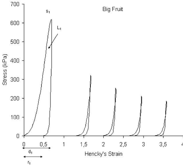
FIG. 5. EXAMPLE OF CYCLIC COMPRESSION/DECOMPRESSION CURVE (BIG FRUIT CANDY)
