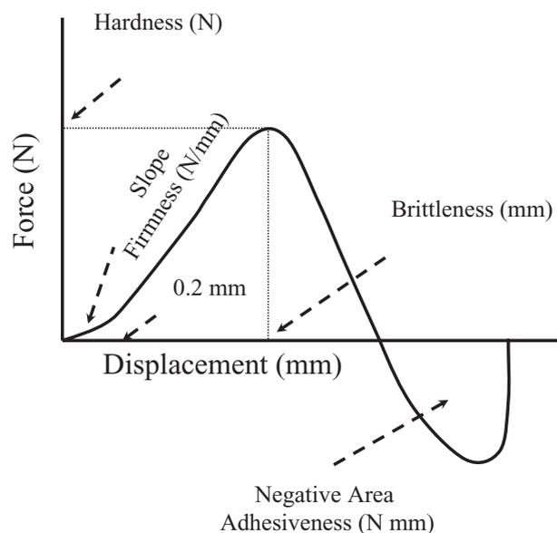
**Fig. 1** Force-deformation curves showing the instrumental textural attributes.
