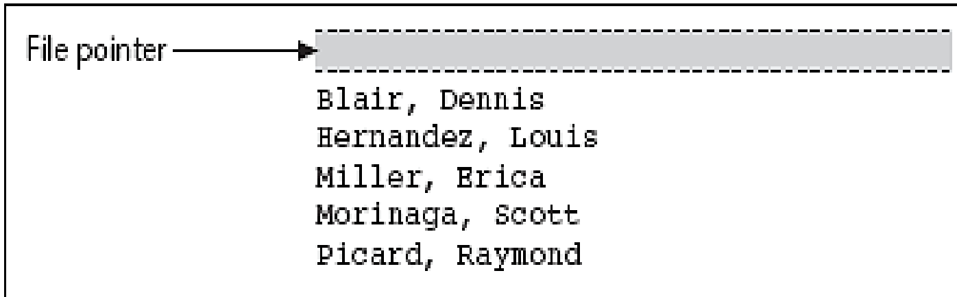
Figure 6-1 Location of the file pointer when the fopen() function uses a mode argument of "r+"
